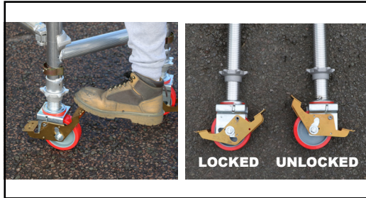
3. Lock Brakes and allow 75mm thread from bottom of castor for levelling
