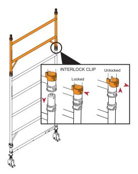
**3** Fit one horizontal brace (red) onto the vertical of a master rung frame as shown, with the claw facing outwards. The frame will now be self-supporting.
