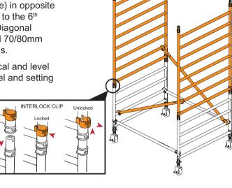
Fit two camlock AGR frames, one on each side of the tower. The lowest claw of the AGR must be fitted to the 6<sup>th</sup> rung of the tower, as shown.
