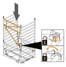
**5.6** Repeat AGR installation steps for the second AGR on the opposite side of the tower, before fitting platforms.
