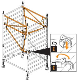
Camlock Advance Guardrail (AGR) Frame Assembly Installation
