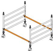
Fit two additional end frames and ensure the frame interlock clips are engaged.
