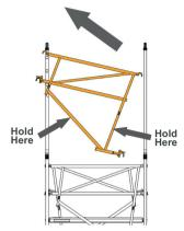
**5.2** With AGR resting on the rung of the end frame, rotate AGR upwards into position shown.
