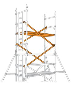
**7** Climb up the inside of the tower and from protected position of the trapdoor, fit guardrails to the 7<sup>th</sup> and 8<sup>th</sup> rungs (in that order) on both sides of the tower.
