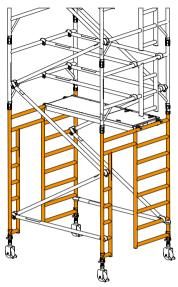
If end walk-through access is required at the base of 2.2m, 4.2m, 6.2m, 8.2m, 10.2m or 12.2m platform height, 1450 wide towers, walk-through frames may be used.
