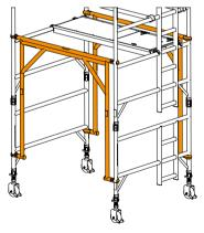
If side walk-through access is required at the base of 4.2m, 6.2m, 8.2m, 10.2m or 12.2m platform height towers, high clearance frames may be used in place of the four lower diagonal braces and two lower horizontal braces.
