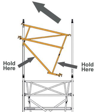
**7.2** With AGR resting on the rung of the end frame, rotate AGR upwards into position shown.
