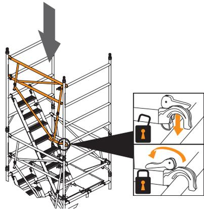
**7.6** Repeat AGR installation steps for the second AGR on the opposite side of the tower, before fitting platforms.
