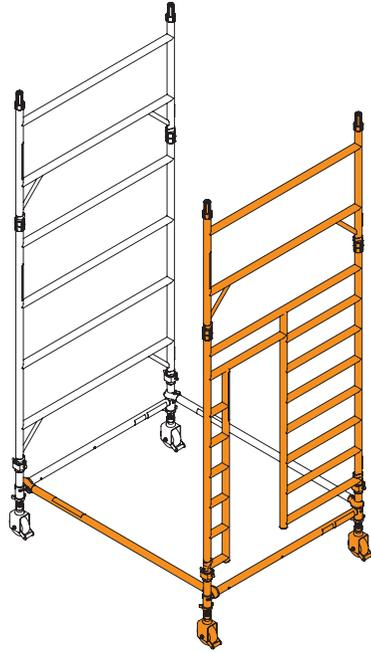
**5** Fit two diagonal braces (blue) in opposite directions, from the 1<sup>st</sup> rung as shown. Diagonal braces should be positioned 70/80mm inboard of the frame verticals.
