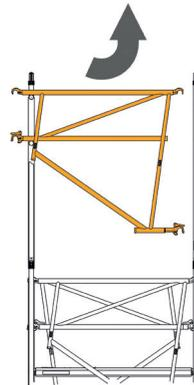
**7.3** Lift AGR to ensure claw latch clears rung of end frame and move AGR across so both top hooks are above top rungs of end frames, as shown.
