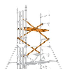
Climb up the inside of the tower and from protected position of the trapdoor, fit guardrails to the 7<sup>th</sup> and 8<sup>th</sup> rungs (in that order) on both sides of the tower.
