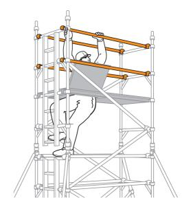
Continue the procedure until the required height is reached, adding additional pairs of end frames, diagonal braces and fitting trapdoor platforms, as shown on previous steps. At every platform level, add horizontal braces as guardrails from the protected position within the trapdoor (as shown in **Step 7**).
