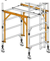
If side walk-through access is required at the base of 4.2m, 6.2m, 8.2m, 10.2m or 12.2m platform height towers, high clearance frames may be used in place of the four lower diagonal braces and two lower horizontal braces.
