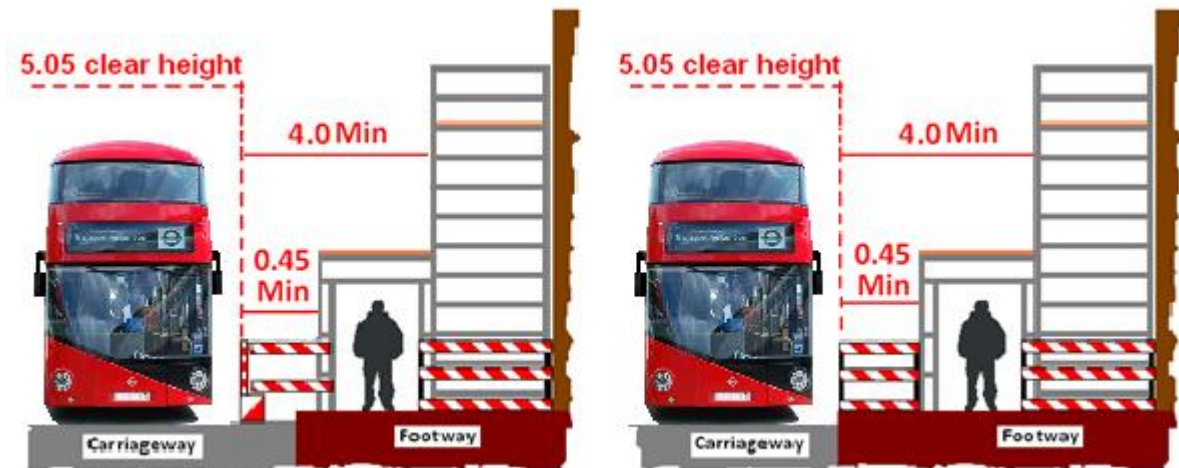
Figure 4 Protection structures and protection zones
