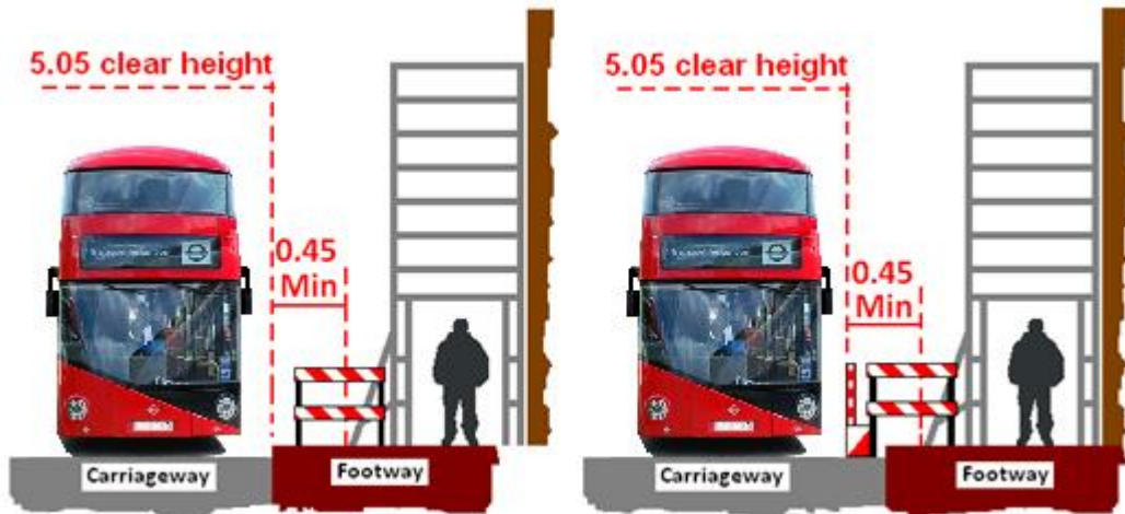
Figure 3a Minimum 0.45 to edge carriageway
