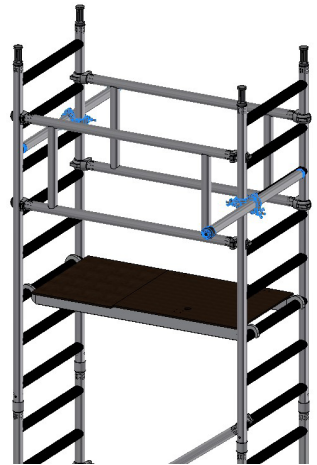
18) Fit a side prop to the top of each frame above the 3rd rung down, one either end of the tower.
