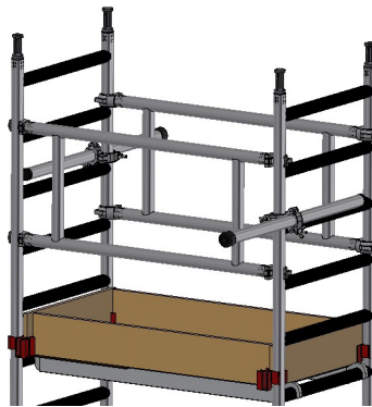
20) Then fit your toe-boards using the clips.
