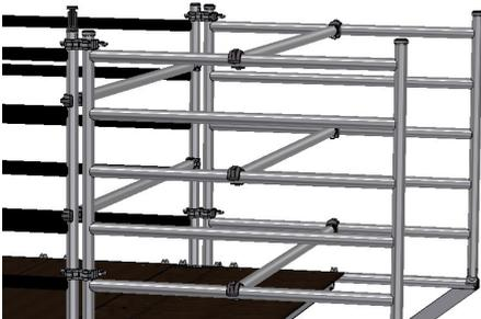
5. Fit an additional set of guardrail braces. This will be 3 horizontal braces hooks facing down to lock onto the cantilever frames.
