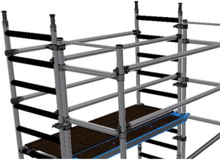
3. From behind the guardrail braces fit the infill platform.
