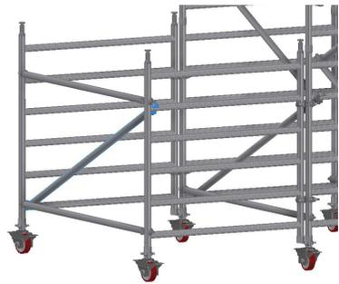
4. Fit 1 diagonal brace to the bottom rung of a buttress frame at the furthest point away from the main tower.
