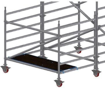
5. Fit ballast platform to the bottom rung at the end away from the main tower structure. Level the buttress using a spirit level as a guide; re-tighten couplers before continuing (if required).
