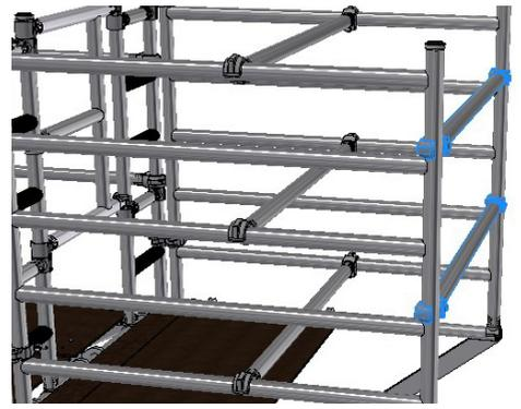
6. Reposition the inner braces to the verticals above the 3rd and 5th rung on the Cantilever frames to complete your working guardrails, hooks facing out.
