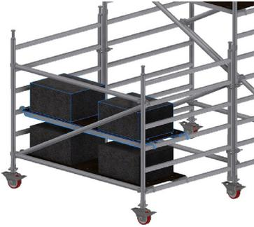
7. All additional ballast platforms and weights must be positioned on the buttress frames only, starting above the first.
