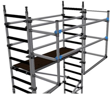
2. From behind the guardrail braces fit 2 more braces to complete a new guardrail.
