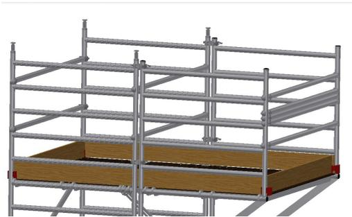
9. Fit toeboard clips and toeboards to complete the structure.
