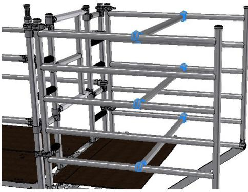
5. From behind the rungs fit an additional set of guardrails on Cantilever frame rungs for the new platform, pushing down to lock on.
