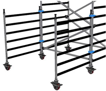
2. Secure each buttress frame to the main tower structure using the approved swivel couplers. 1 above the top rung and 1 above the second rung on each side.
