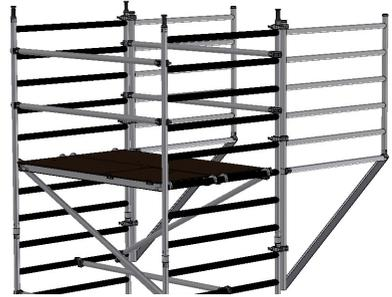
2. Fit cantilever frames; ensure the rungs line up to avoid trip hazards on the platform decks. Ensure couplers are tight. Repeat on the opposite side.
