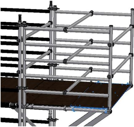
7. From behind the inner set of guardrails fit a platform next to the one you are on. Go to Step 9
