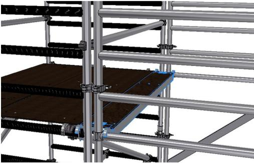
3. From behind the guardrail braces fit the infill platform.
