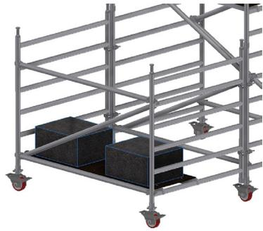
6. Fit the required ballast weight evenly on the ballast platform(s) and secure in place.
