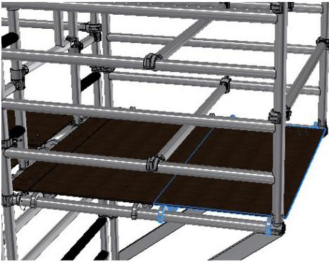
7. Going through the rungs or gate, from behind the new guardrails fit a platform next to the one you are on.
