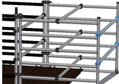
6. Reposition the inner braces to the verticals above the 3rd and 5th rung on the Cantilever frames to complete your working guardrails, hooks facing out. (Single Width Cantilever go to step 8)
