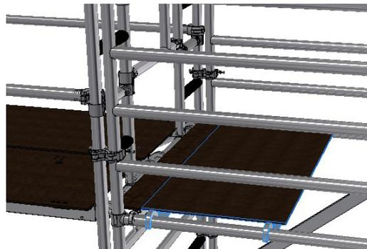
4. From behind the rungs fit a platform on the nearside of the cantilever system next to the end infill platform. (Single Width Cantilever go to step 7)
