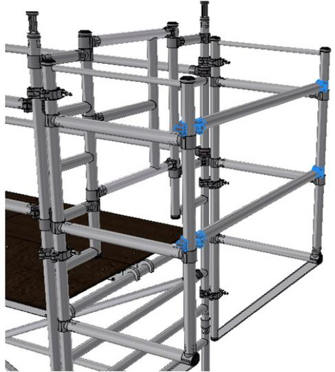
1. Fit 6 swivel couplers to your tower as seen above. Fit cantilever frames; ensure the rungs line up to avoid trip hazards on the platform decks. Ensure couplers are tight. Repeat on the opposite side.
