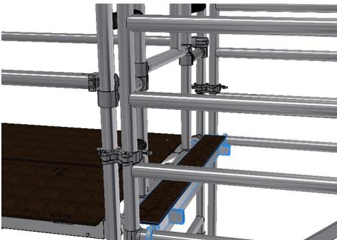
3. From behind the gate fit the end infill platform.
