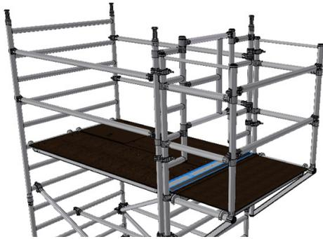
5. From behind the gate fit the cover panel over the platform hooks.
