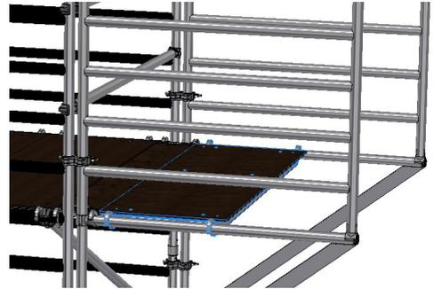
4. From behind the guardrail braces fit a platform next to the infill platform. (Single Width Cantilever go to step 6)
