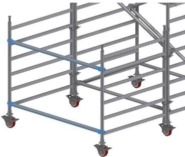
3. Fit 1 buttress horizontal brace to the vertical above the 5th rung and 1 above the bottom rung at the end away from the main tower structure.
