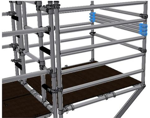
8. Reposition the inner set of braces to store ready for safe dismantling on the tower. (Double Width Cantilever only)
