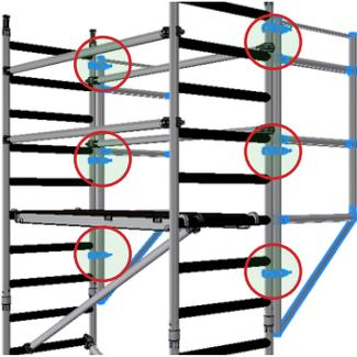
1. Fit 6 swivel couplers to the vertical as seen above. Ensure they are evenly spaced out. 2. Fit cantilever frames; ensure the rungs line up to avoid trip hazards on the platform decks. Ensure couplers are tight. Repeat on the opposite side.
