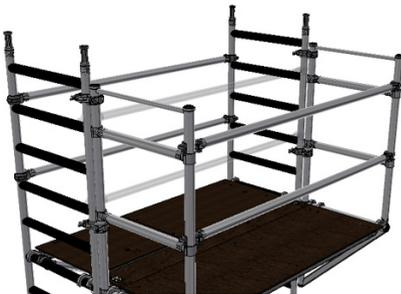
5. You can now remove your original guardrail braces from the tower leaving the new cantilever guardrail braces
