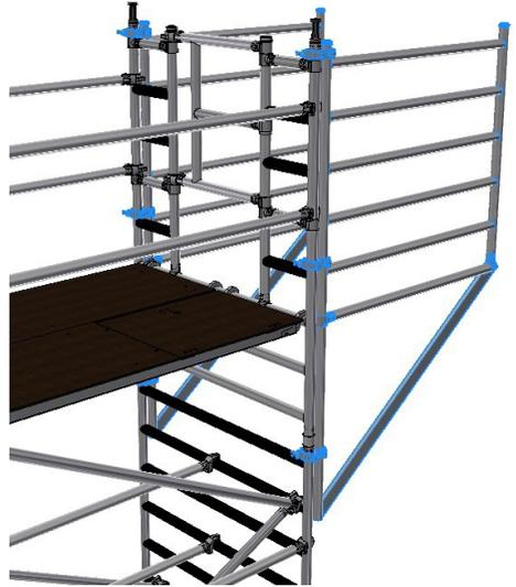
2. Fit cantilever frames; ensure the rungs line up to avoid trip hazards on the platform decks. Ensure couplers are tight. Repeat on the opposite side.
