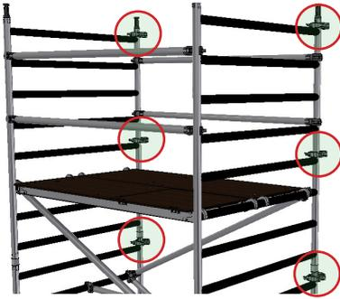
1. Fit 6 swivel couplers to the vertical as seen above. Ensure they are evenly spaced out.
