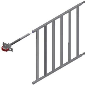
1. Insert castor and leg into each of the buttress frames and lock brake when in position. See image on page 12 for castor brake operation.
