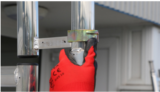
6. After adding frames, always remember to engage all your interlock clips.
