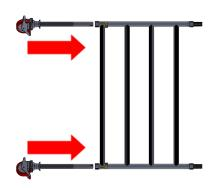
Attach one horizontal brace to the second rung of the end frame, claws facing downwards.
