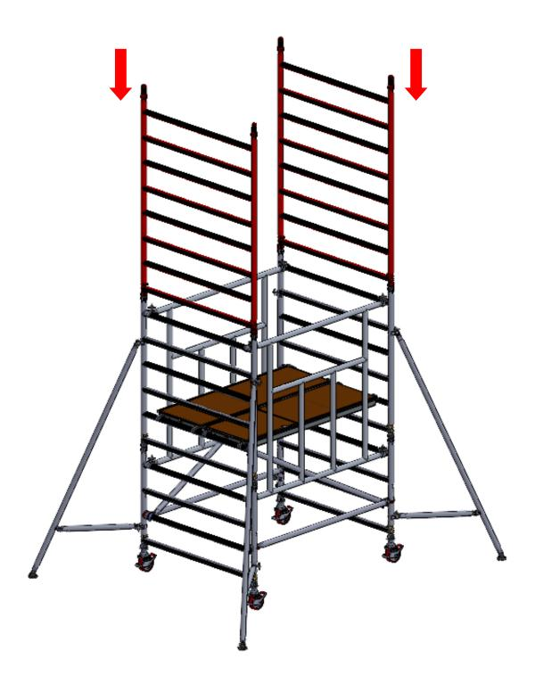
7. Fit a AGR on each side of the tower. The bottom of the AGR must be fitted to the 2nd rung of the 8 rung sides, as shown. The AGR should be placed up against the end frame verticals. Make sure bottom AGRs are locked before you climb tower. (refer to page 9)
