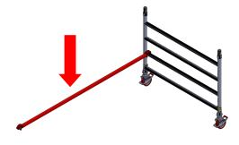
end of the horizontal brace to the second end frame. Now connect the frames using a second horizontal brace on the opposite side, attach inside of the rung frame just above the second rung, claws facing outwards, this will square the tower.
