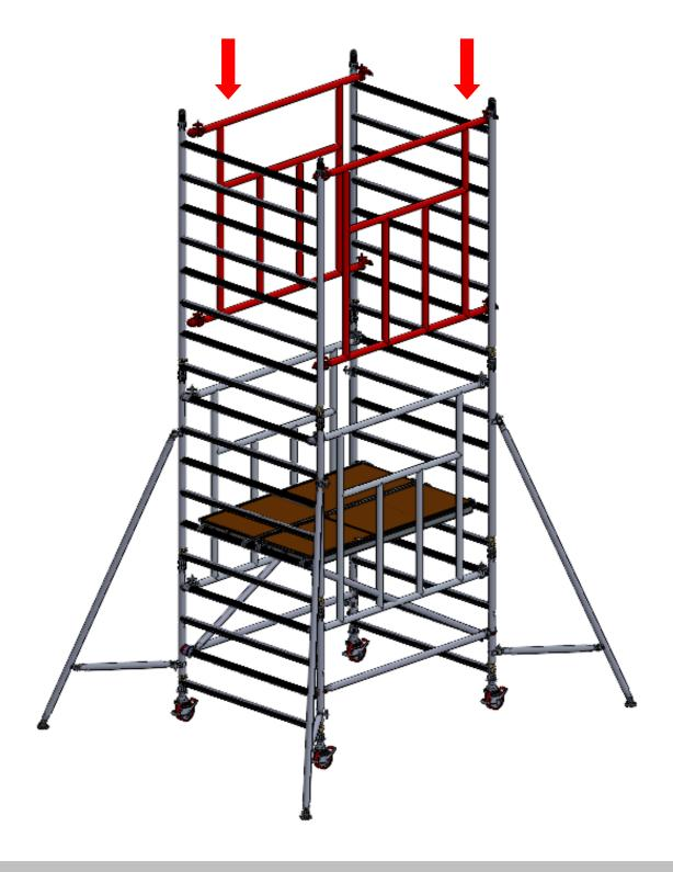
Place a trap door platform and a fixed platform on the 4th rung of the 8 rung frame, ensure the trap door platform is on the ladder side of the structure.
