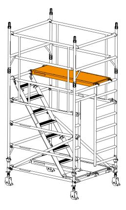
9 Fit stabilisers (see notes on **page 8**). Telescopic stabilisers must always be fully extended.
