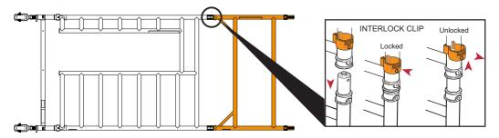
Fit one horizontal brace (red) onto 3 the vertical of the span frame assembly, just above the bottom rung of the master rung, with the claw facing outwards. Lock castors. The frame will now be self-supporting.
