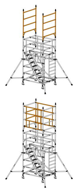
**12** Standing on the fully guardrailed platform, fit the next staircase above and aligned with the first staircase with the landing claws fitted to the top cross member of the walk-through frame as shown.
