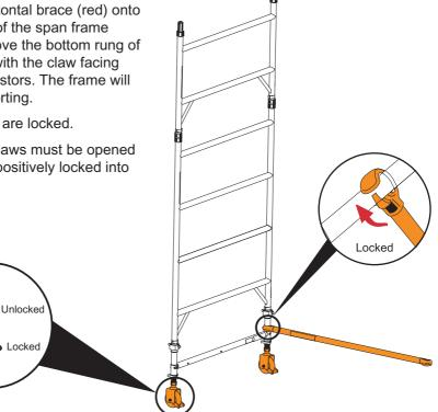
Position walk-through frame assembly as shown and fit the other end of the horizontal brace onto the vertical, just above the bottom rung.
