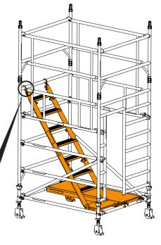
**8** Fit a fixed platform to the top rung of the walk-through frame, directly above the lower fixed platform. Ensure the platform wind-locks are engaged.
