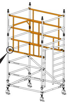
**7** Position a fixed platform next to the diagonal brace as shown. Fit the staircase unit between the master rung and the top cross member of the 4 rung span frame. Ensure that the staircase claws are positioned outside of the datum rivets on the master rung as shown and the staircase is aligned with the opening in the frame.
