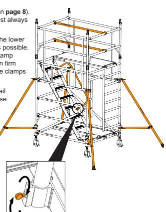
**10** Standing on the fully guardrailed platform, fit two 4 rung span frames in positions shown.
