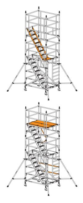
**14** Fit toe board holders and toe boards around the edges of the top platforms as shown.
