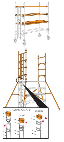
Fit two pairs of diagonal braces in opposite directions between the 3<sup>rd</sup> and 5<sup>th</sup> rungs and the 5<sup>th</sup> and 7<sup>th</sup> rungs.
