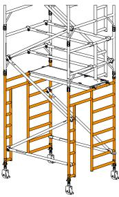
If side walk-through access is required at the base of 4.2m, 6.2m, 8.2m, 10.2m or 12.2m platform height towers, high clearance frames may be used in place of the four lower diagonal braces and two lower horizontal braces.
