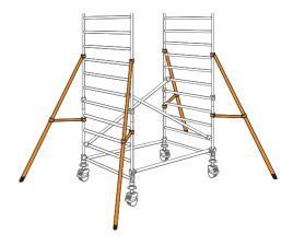
Fit the next pair of diagonal braces in opposite direction between the 6th and 10th rungs. Fit a trapdoor platform on the 8th rung (2.0m) on one side of the tower. Ensure that the trapdoor is positioned with the hinges towards the outside of the tower as shown.
