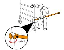
Position the second end frame as shown and at the other end of the horizontal brace onto the vertical, just above the bottom rung.
