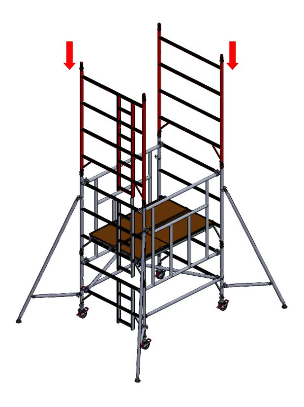
7. Fit a AGR on each side of the tower. The bottom of the AGR must be fitted to the 1st rung of the 4 rung sides, as shown. The AGR should be placed up against the end frame verticals. Make sure bottom AGRs are locked before you climb tower. (refer to page 9)
