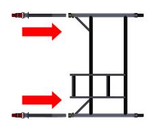
Attach one horizontal brace to the bottom rung of the span frame, claws facing downwards.
