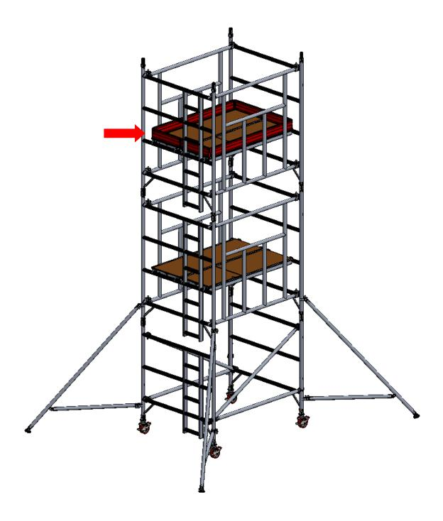
Maximum distance between platforms should not exceed 2.25m. Maximum distance to first platform should not exceed 3.4m
