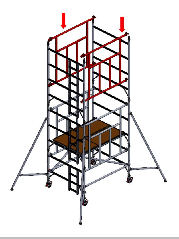
Place a trap door platform and a fixed platform on the 2nd rung of the 4 rung frame, ensure the trap door platform is on the ladder side of the structure. LOCK WIND LOCKS.
