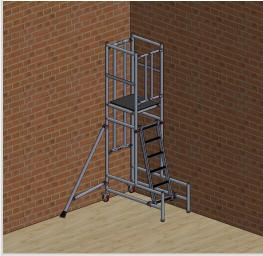
4. In open area, working at rear or overhead, put stabilisers at 45° from body as shown in picture.
