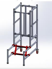
5. Hook on platform at chosen height and turn wind lock to closed position.
