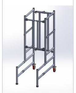
3. Ensure the bottom locking elbow has engaged.
