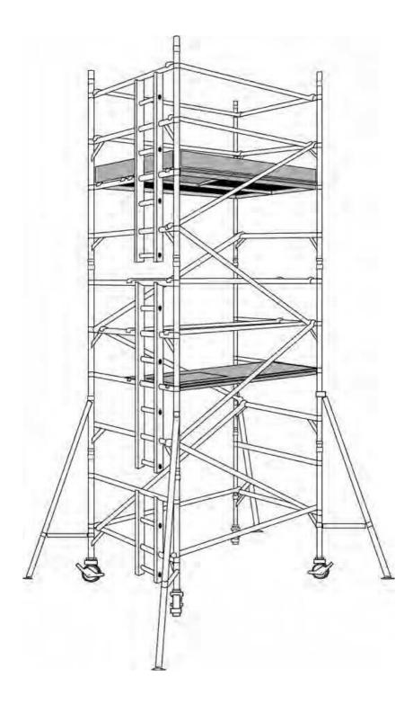
When building structures over 4.2 metres remove platform and 4 horizontol braces fromplatform height at 2.2 meters and use to complete structure.
