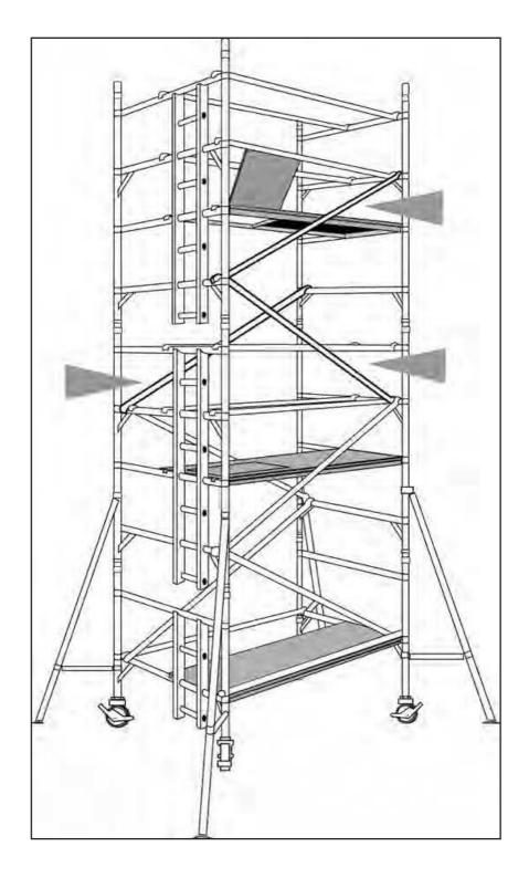
Fit the final diagonal braces as shown. This stage will provide a platform
