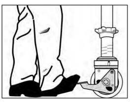
Press to engage — lift to disengage.
