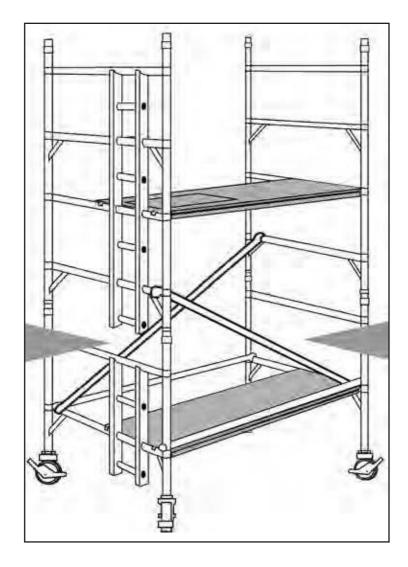
\*Platform can be placed at bottom of tower if required. As shown in diagram
