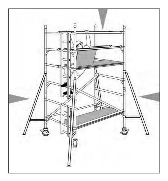
6 Attach 2nd pair of diagonal braces following on from the previous ones. Attach the next 4 rung frames and lock clips (as per fig. 6).
