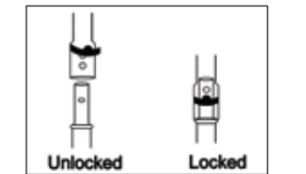
2)Snap pins - Unlock the interlock Clips on all frames. When installed, always move the interlock clip to the "Locked" Position.
