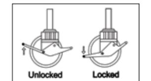
4)Wheel lock - Install castor / leg assembly to frame by pushing the leg into the frame tube. This Should be done with manual force only, no tools. Lock Castors before ascending any part of the tower.
