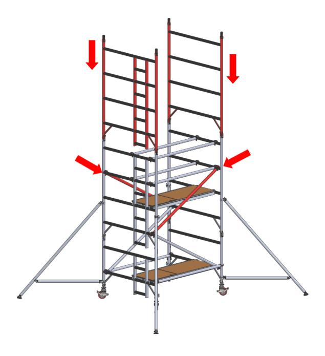
7. If completing the tower at this height (4m), continue with step 8. When building beyond this level, repeat steps 4, 5 and 6 until desired level is achieved, then complete the tower with steps 8 and 9. Reuse the trap door platform from 1st rung on the final height.
