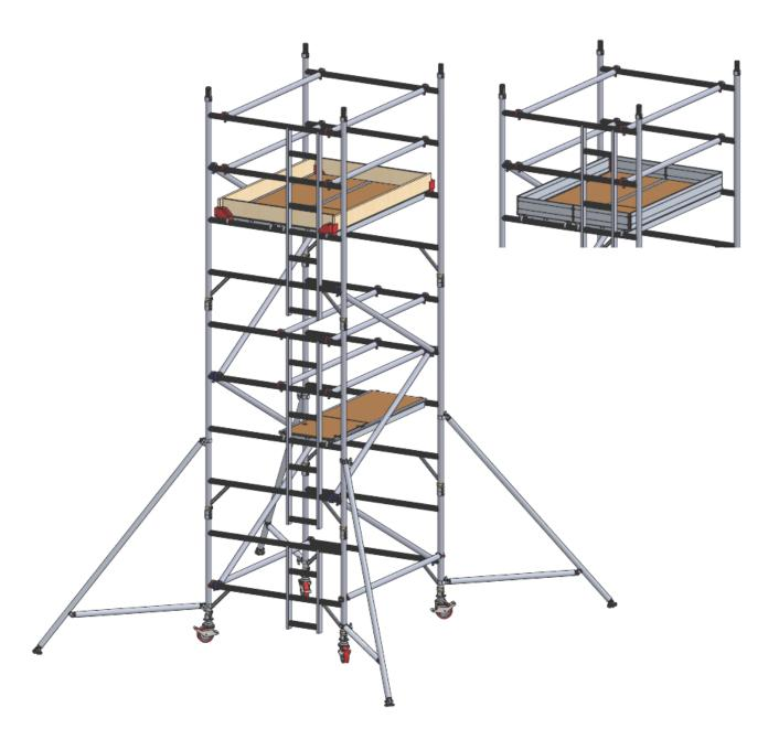
Maximum distance between platforms should not exceed 2.25m. Maximum distance to first platform should not exceed 3.2m
