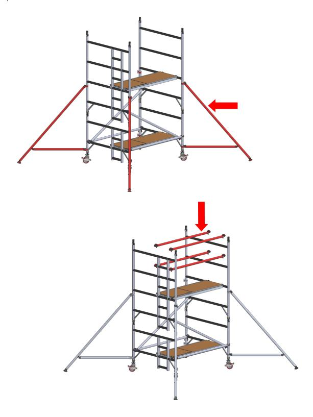
Attach 2nd pair of diagonal braces following on from the previous ones. Attach the next 4 rung frames and lock clips (as per fig. 6).
