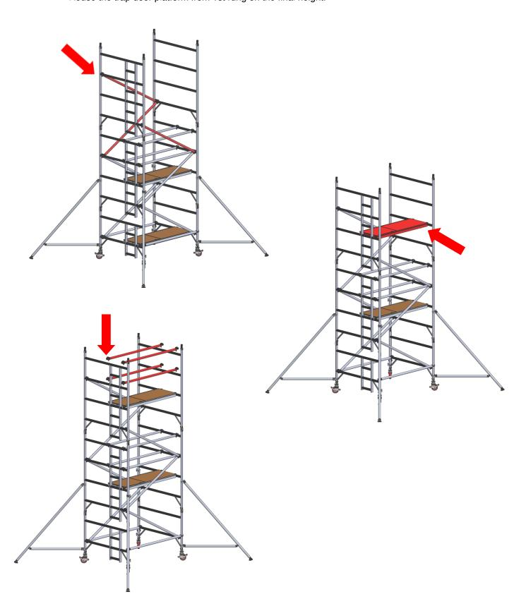
Fit the final diagonal braces as shown. This stage will provide a platform height of 4m. Attach diagonal braces as per fig. 7. The 1st rung trap door platform should be moved up to the 8th rung, the fixed platform can now be fitted alongside it.
