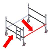
Insert 4 rung frames to correspond with the 2 rung frames (fig. 3) and lock the locking clips (refer to page 8).
