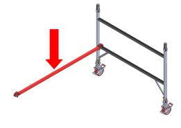
other end of the horizontal brace to the ladder frame. Now connect the frames using a second horizontal brace on the opposite side, attach from the inside of the frame just above the bottom rung, claws facing outwards, this will square the tower.
