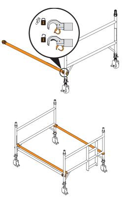
NOTE: This tower does not use the standard BoSS diagonal cross bracing system. Diagonal braces are fitted parallel.
