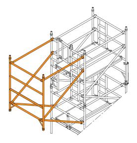
11 From the protected position within the main tower, fit two fixed platforms. Fit two horizontal braces in positions shown. Ensure all wind-locks are engaged. Ensure all claws are positively locked into position.
