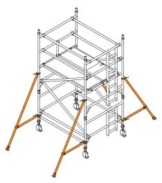
Fit two castors with adjustable legs to the 4 rung span frame and link to the main frame using 1.8m horizontal braces and 2.1m diagonal braces. Fit fixed platforms as shown to support ballast, refer to tables on page 13.
