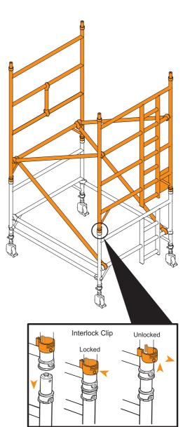
Fit the trapdoor platform and fixed platform on the 4<sup>th</sup> rungs of the tower, ensuring the platforms are positioned each side of the 0.5m vertical brace as shown. The trapdoor platform must be oriented such that the trapdoor opens towards the outside of the structure. Ensure the platform wind-locks are engaged.
