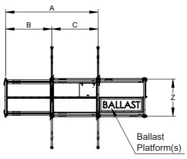
the castors, is not exceeded. Use good manual handling techniques when handling ballast. See quantity schedule on pages 8 to 11 for ballast information.
