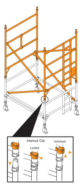
Fit the trapdoor platform and fixed platform on the 4<sup>th</sup> rungs of the tower, ensuring the platform are positioned each side of the 0.5m vertical brace as shown. The trapdoor platform must be oriented such that the trapdoor opens towards the outside of the structure. Ensure the platform wind-locks are engaged.
