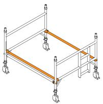
Fit the 0.5m vertical brace into a span frame between the 2<sup>nd</sup> and 3<sup>rd</sup> cross bars at mid span.
