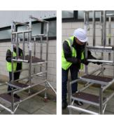
Add the additional brace below the platform. For a the step platforms and stepfold 2 you should now the ribbed brace. Then have 2 ribbed braces below the working
