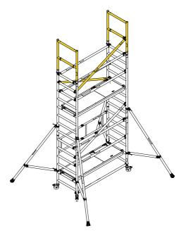
Reposition trapdoor decks and horizontal braces.
