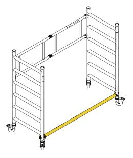
Fit 2 rung guardrail frames as shown. Fit diagonal brace in position shown.
