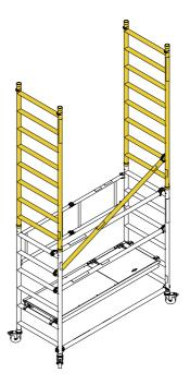
**5** Fit trapdoor deck as shown. From the protected trapdoor position, fit horizontal braces as shown.
