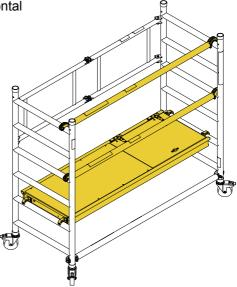
Fit 8 rung frames as shown. Fit diagonal brace in position shown.
