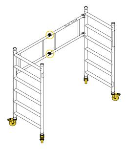
Fit horizontal brace in position shown. Check tower is square and level.
