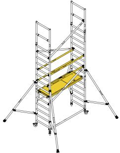
Fit the trapdoor deck as shown. From the protected trapdoor position, fit horizontal braces as shown.
