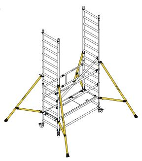
6 Fit trapdoor deck as shown. From the protected trapdoor position, fit horizontal braces as shown.
