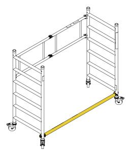
Fit trapdoor deck and horizontal braces in position shown.
