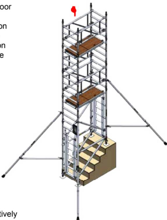
**13** Unclip storage strap from aluminium folding toe board set, unfold and fit into position on working platform.
