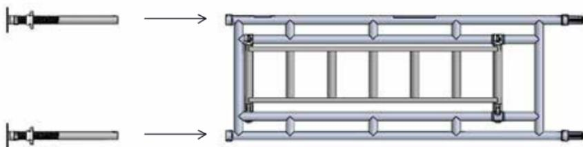
**2** Fit one horizontal brace (red catch) onto the vertical of end frame on the climbing side in position indicated with an arrow, with the claw facing outwards. Ensure the gate opens as shown.
