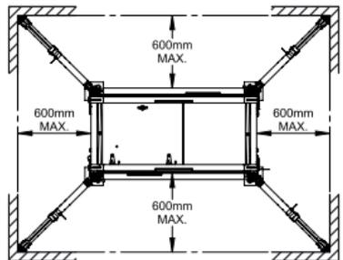
Attach one confined space stabiliser to each corner of the tower as shown (see page 18). Ensure stabiliser feet are touching the lift shaft walls - adjust confined space stabilisers as necessary to achieve this.
