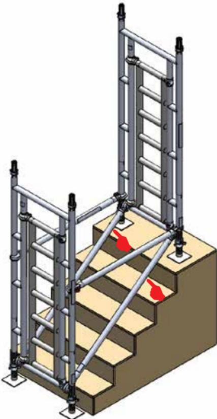
**4** Fit two diagonal braces (blue catch) between bottom rungs of both portal ladder frames, one on each side of the tower. Claws must face downwards. The structure must be vertical to within 1cm per metre.
