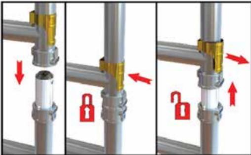
Ensure interlock clips on frame members are in the 'locked' position.
