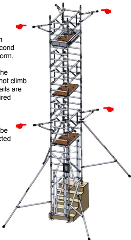
Ensure the end of the stabiliser arm contacts the wall. If it does not, adjust by unclipping and extracting the locking pin, sliding the arm until correct length and hole alignment is achieved. Reinsert the locking pin, ensuring clip is engaged. See images below:
