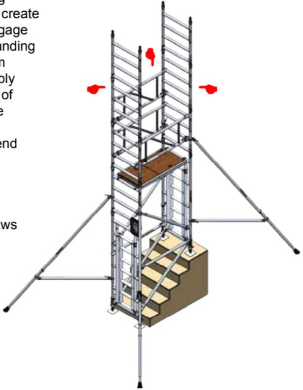
**11** Fit one 1.3m trapdoor deck onto the eighth rung above the platform deck as shown. Ensure wind-locks are engaged.
