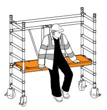
**5** Climb onto the platform in the sequence shown. From the seated position, fit horizontal braces as guardrails on the 5th and 7th rungs on the open side of the base unit. Do not stand on the platform until the guardrails are in place.
