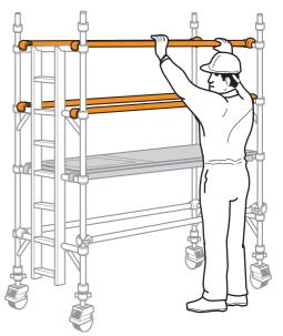
Fit two diagonal braces in opposing directions between the 1st and 3rd rungs. Ensure that the frames are vertical and level by checking with a spirit level and setting the adjustable legs as necessary. Fit stabilisers (see notes on page 9). Fit the next pair of end frames and check the frame interlock clips are engaged.
