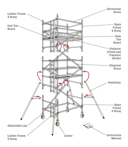
BoSS 1450 Ladderspan to EN 1004: Available in 2 lengths - 1.8m and 2.5m
