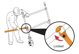
Position the ladder frame as shown and fit the other end of the horizontal brace on to the vertical (just above the bottom rung). Fit a second horizontal brace between the bottom rungs on the other side of the frames to square the tower.
