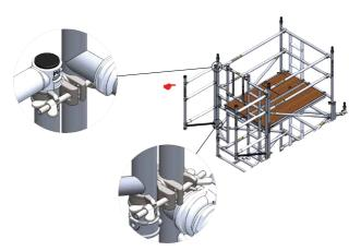
11 From the protected position within the main tower, fit the cantilever end beam unit. Ensure the claws touch on the ring.
