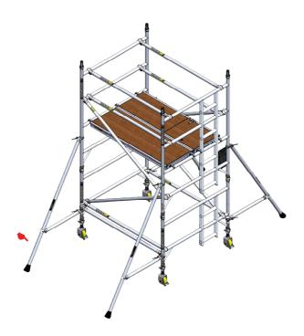
Fit two castors with adjustable legs to the 4 rung span frame and link to the main frame using 1.8m horizontal and 2.1m diagonal braces. Fit fixed decks as shown to support ballast, refer to tables on page 25. Level the whole assembly and ensure castors are locked. Ensure all wind-locks are engaged.
