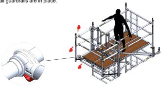
Fit the 0.3m and 0.6m infill decks. Fit toe board holders and toe boards around edges of top decks, as shown. Store the guardrail frame at the base of the tower as shown.
