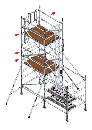
10 Fit two cantilever frames, as shown. Note position of couplers. Ensure wing nuts are fully tightened.
