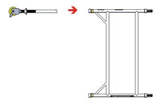
Fit one horizontal brace (red catch) onto the vertical of the 2 rung span frame, just below the bottom rung with the open section of the claw facing outwards.
