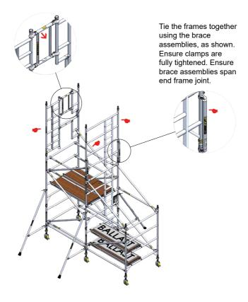
Fit the fixed deck and trapdoor deck 2.0m above the previous level. Ensure all wind-locks are engaged. Note the orientation of the trapdoor. From the protected trapdoor position, fit guardrails at 0.5m and 1.0m (in that order) above the platform level. Fit two diagonal braces in positions shown. Fit two 1.45m horizontal braces to span frame, 0.5m and 1.0m below step-through multi-purpose ladder frame as shown.
