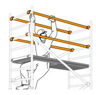
Continue the procedure until the required working height is reached, adding additional pairs of end frames, diagonal braces and fitting trapdoor platforms, as shown on previous steps. At every platform level, add horizontal braces as guardrails at 2 and 4 rungs above the platform (in that order) on both sides of the platform (as shown in **Step 5**).
