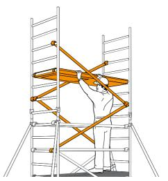
Climb up the inside of the tower and from the protected position of the trapdoor, fit horizontal braces as guardrails (on both sides) to the 14<sup>th</sup> and 16<sup>th</sup> rungs (2 and 4 rungs above the platform in that order).
