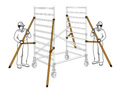
Fit a temporary deck on the lowest rungs. Fit a trapdoor deck on the 8th rung (2.0m) on one side of the tower. Ensure that the trapdoor is positioned with the hinges towards the outside of the tower as shown. Climb the end frame below the trapdoor on the
