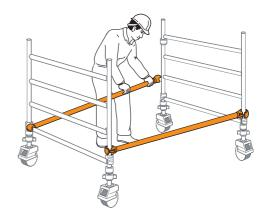
Fit two additional end frames and check that the frame interlock clips are engaged. Fit two diagonal braces (blue) in opposing directions between the 2<sup>nd</sup> and the 6<sup>th</sup> rungs. Ensure the frames are vertical and level by checking with a spirit level and setting the adjustable legs as required.
