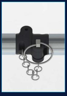
Once the podium has been unfolded, locate and lock in the bottom and top pins on the horizontal bracing at the back of the podium as shown in the diagram. If the top pin is inaccessible from the ground, lock in the top pin when the podium is fully assembled and accessed for the first time. There is no safety risk when doing this as the deck, ladder frame and bottom pin keeps the podium secure and free from any movement.
