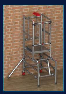
If you are positioning the LytePOD with the rear elevation against a surface/wall or are applying a lateral force from the back of the podium, position both stabilisers at a 90 degree angle which is perpendicular to the podium. Fully tighten up the clamps on each stabiliser and ensure both are secure.
