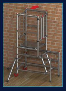
If you are positioning the LytePOD with a side elevation against a surface/ wall or are applying a lateral force from the side of the podium, position one stabiliser at a 90 degree angle which is perpendicular to the podium and the other stabiliser parallel to the surface/wall. Fully tighten up the clamps on each stabiliser and ensure both are secure.
