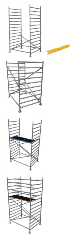
4. Attach an 8 rung DW frame on top of the 6 rung DW frames, Ensure the interlock clip is engaged on all frames.
