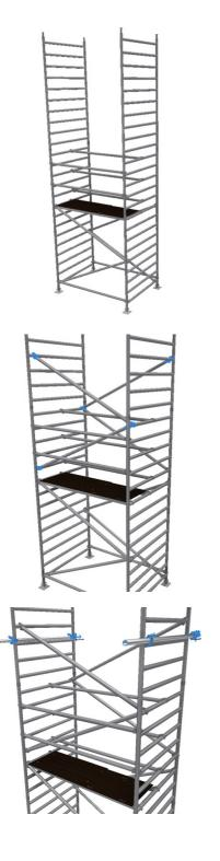
8. Attach a 10-rung frame above the 8-rung frame.
