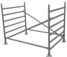
3. Hold another 6 rung DW frame (with legs and base plates) upright and attach 2x horizontal braces above the first rung of the frame as before. Ensure the "kliker" is fully engaged.
