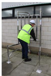
Open the unit on a firm and level base, lock the folding section and then lock the wheels.
