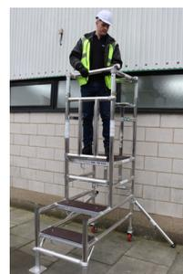
Access the platform using the step platforms and the ribbed brace. Then close the gate and fit both guardrail braces.
