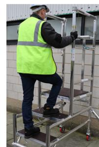
When descending from the platform, use the step platform up 1 rung.
