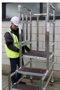
Fit the working platform on the 3rd rung for the stepfold podium 1 or 4th rung for podium 2.
