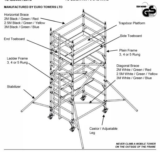
MAX SAFE WORKING LOAD FOR TOWER 750KG (including self-weight)
