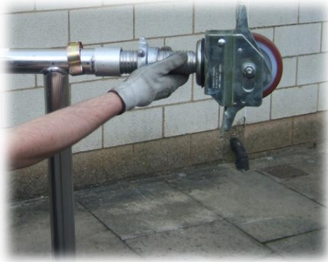
Insert Castors and adjustable legs into frames.
