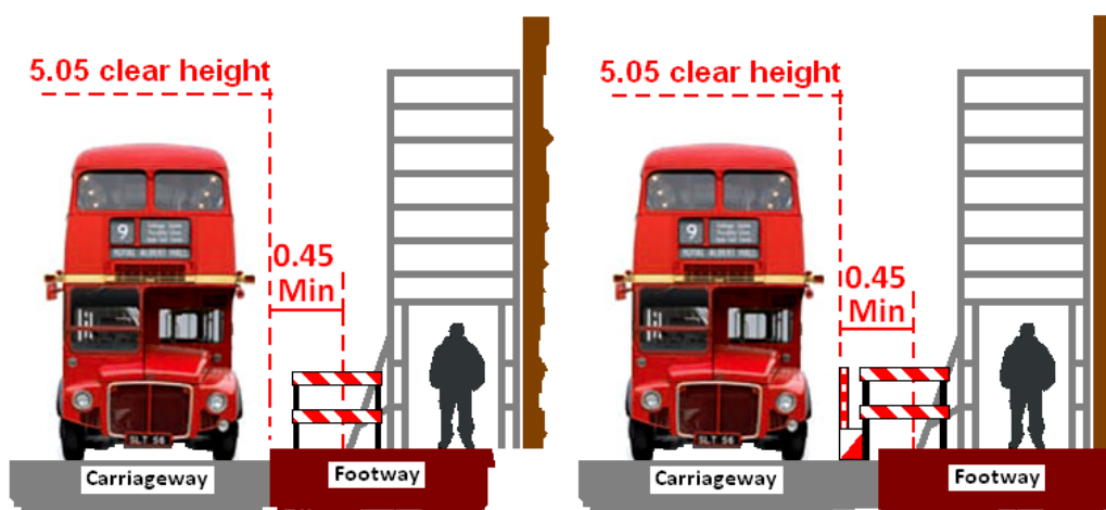
Figure 3a Minimum 0.45 to edge carriageway
