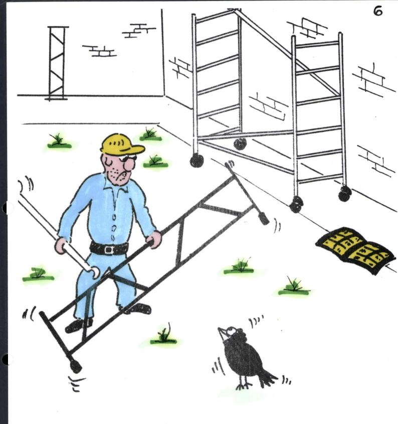
CHECK THAT ALL COMPONENTS ARE OF THE SAME MAKE AND CORRECT TYPE AND THAT THE CORRECT NUMBER ARE ON SITE.
