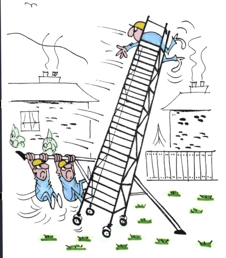
INSPECT BEFORE EACH USE TO SEE THAT HEIGHT TO BASE RATIO IS WITHIN LIMITS. RAISE STABILISER FEET NOT MORE THAN 1/2" ABOVE GROUND WHEN MOYING,
