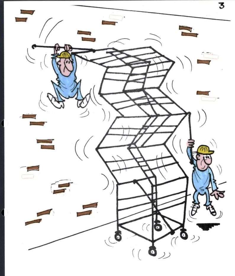
BRACING MEMBERS SHOULD BE FITTED IN ACCORDANCE WITH SUPPLIER'S INSTRUCTIONS.
