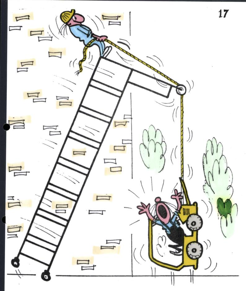
IF POSSIBLE HOIST ANY LOADS INSIDE THE TOWER, WHEN RAISING LOADS OUTSIDE THE TOWER STABILITY IS REDUCED.
