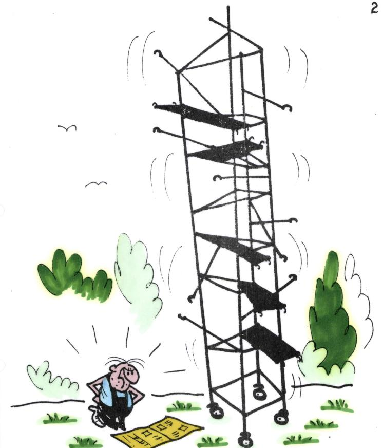
CHECK THAT THE TOWER IS SOUARE 8 VERTICAL & THAT THE HORIZONTAL BRACES & PLATFORMS ARE LEVEL.
