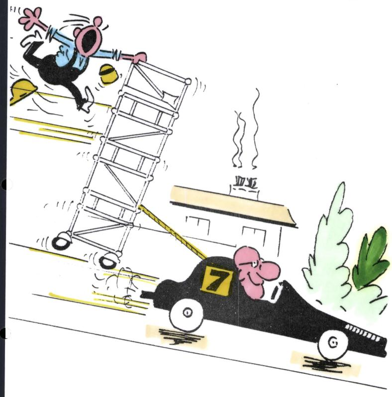
AVOID MOVING THE TOWER BY MECHANICAL MEANS SUCH AS TOWING WITH A VEHICLE
