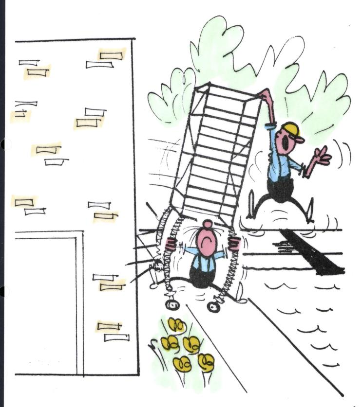
ADJUSTABLE LEGS MUST NOT BE USED AS A MEANS OF GAINING ADDITIONAL HEIGHT.
