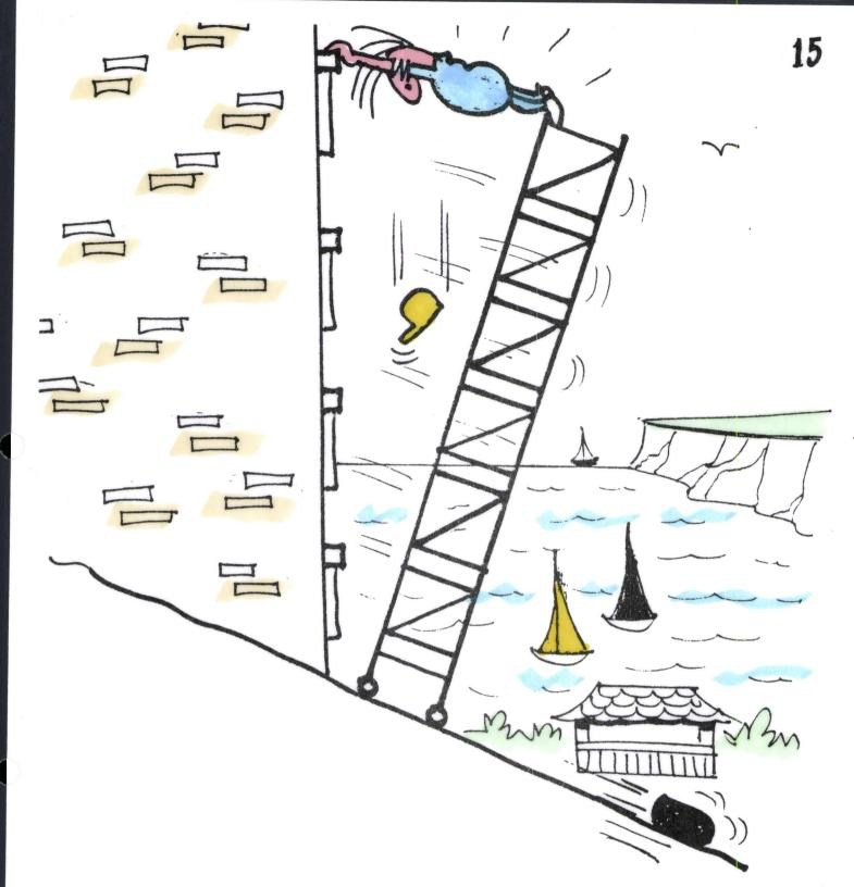
TOWER MUST NOT BE USED ON SLOPING SURFACE WITHOUT ATTENTION TO VERTICAL ALIGNMENT AND STABILITY.
