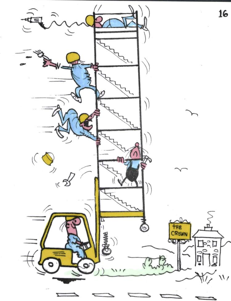
ENSURE THAT MEN AND MATERIALS ARE OFF THE TOWER WHEN MOVING NEVER MOVE THE TOWER WITH FORK LIFT TRUCK
