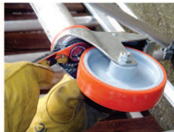
Fig. 2 – detail of castor tightening
